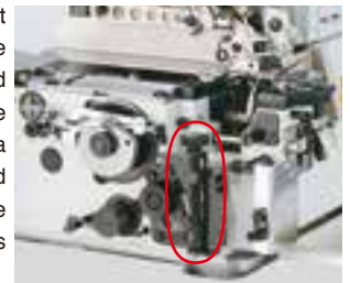
Differential-feed micro-adjustment mechanism
